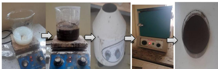
Figure 1 Collagen-based silver nanoparticle synthesis process
