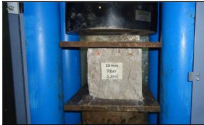
Figure 10 Jute fiber reinforced Composite concrete specimen after compression failure (66).
