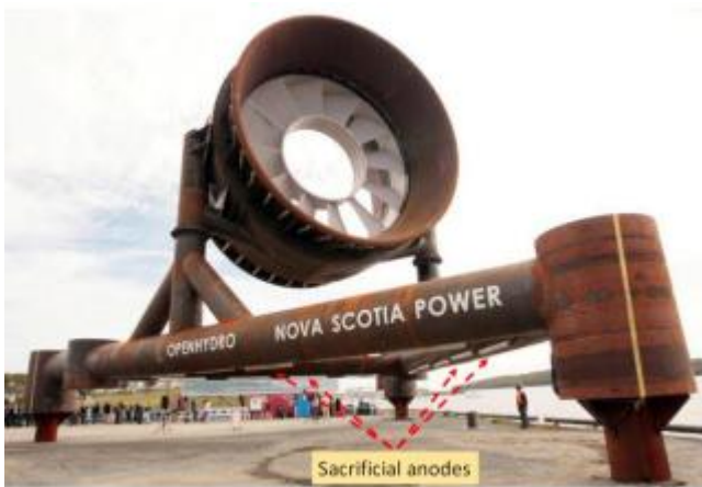
Figure 12 Support structure for Open Hydrokinetic turbine with sacrificial anodes (15)
