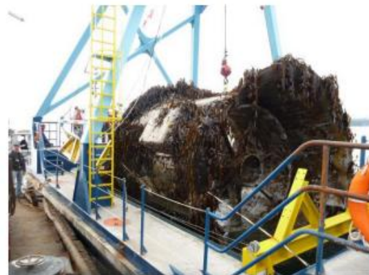
Figure 11 A TidGen turbine in Eastport, Maine, North America, has become fouled (41)
