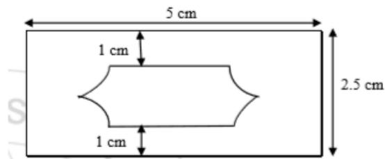
**Figure 5 Dumb bell for tear strength**
