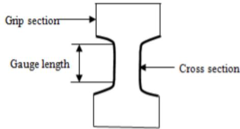
**Figure 4 Dumb bell shape for tensile strength**
