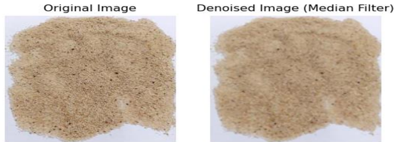
Figure 2: Noise removal using median filtering
