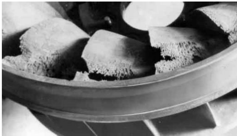
Figure 6. Cavitation damage at the discharge side of the HK turbine blade (23)
