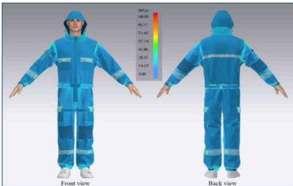
Figure 8. Pressure Distribution of Emergency Rescue Protective Clothing
