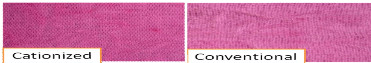
Figure 3 Dyed samples of Cationized and Conventional (using salt)
