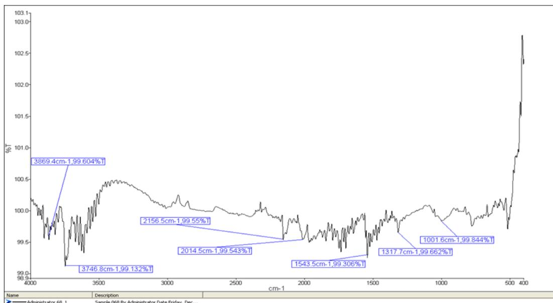
Figure 4: FTIR Analysis of untreated fiber
