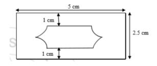
Figure 5 Dumb bell for tear strength
