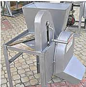
Figure 2: Cassava manual chipper
