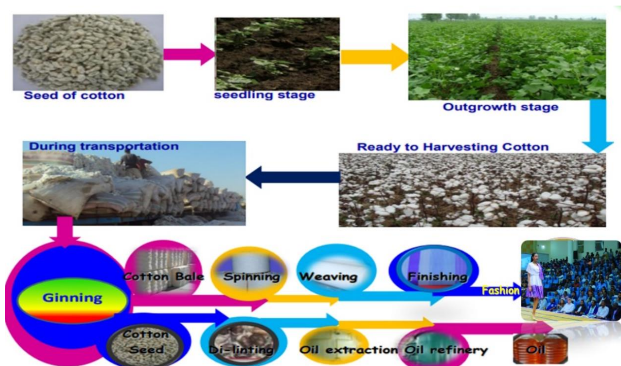
Figure 3. Schematic showing of cotton fiber production processing chain
