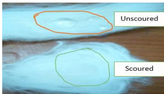
Figure 2: Absorbency of fiber before scouring The absorption rate is increased by scouring the removal of natural impurities to change from
