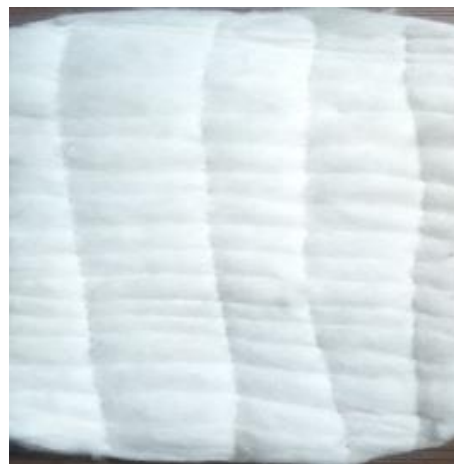
Figure 7: Stich bonded absorbent pad
