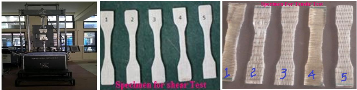
Figure: 1 Universal testing machine (UTM) and specimen Hybrid Sisal-Glass Reinforced HDPE Composite.
