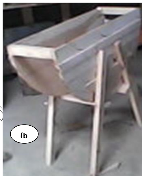
Fig 1: (a) Drawing for groundnut decorticator, (b) photo of the groundnut decorticator during construction
