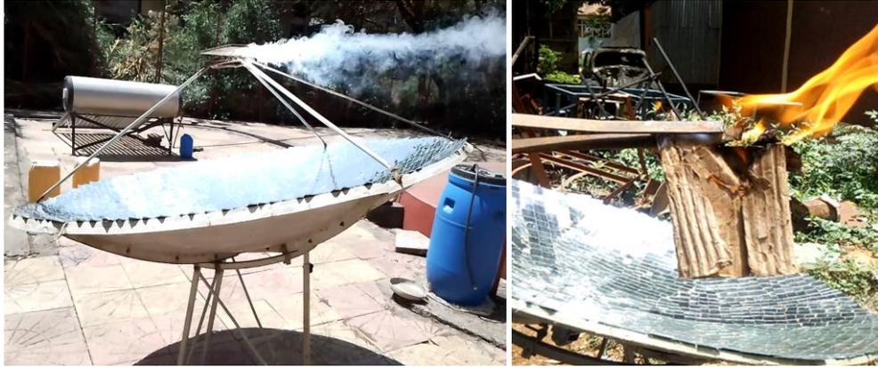
Fig. 2. Parabolic dish with mirror glass reflector.
